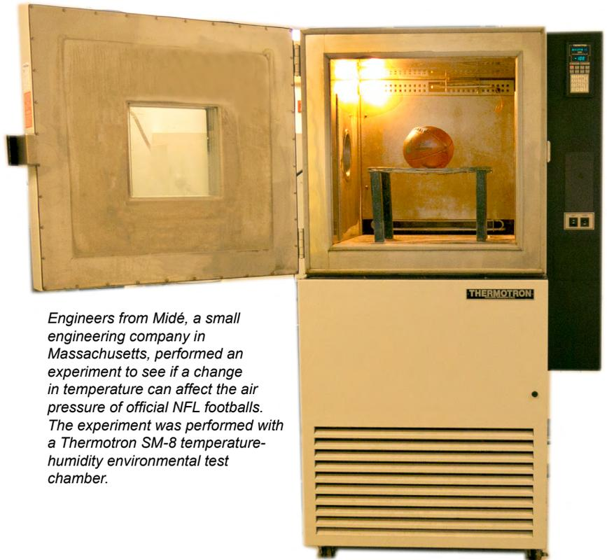
*Engineers from Midé, a small engineering company in Massachusetts, performed an experiment to see if a change in temperature can affect the air pressure of official NFL footballs. The experiment was performed with a Thermotron SM-8 temperature-humidity environmental test chamber.*
