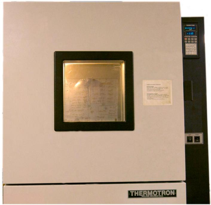
*Two official NFL footballs were placed in Midé's Thermotron SM-8 chamber. They were first conditioned to 24°C (75°F) and measured for air pressure, then the chamber turned down to the gametime temperature of 10°C (50°F) for 90 minutes and then measured the air pressure again.*
