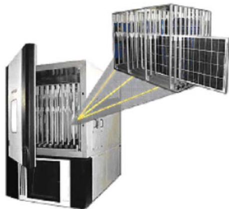
Environmental test chamber with fixtures and solar panels, ready for testing
