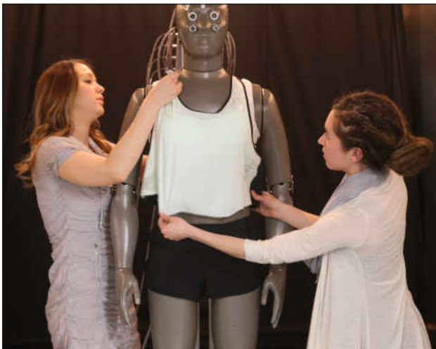
Two faculty members prepare a Thermal Manikin for a temperature and humidity environmental test in the Thermotron Walk-In Chamber.
