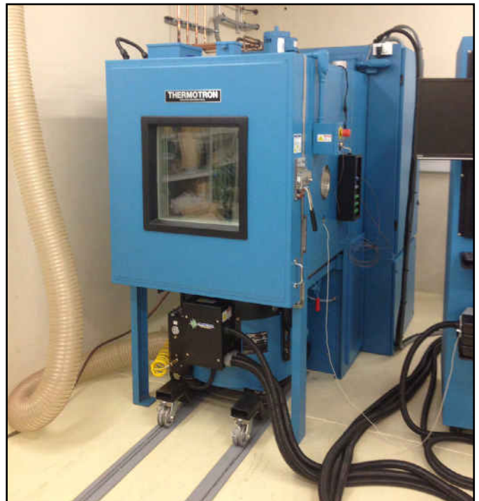
Sat-Com Mechanical Engineering Manager, Glen Brown, bought their chamber-electrodynamic shaker combined system from Thermotron because they are a single-source supplier, ensuring that the equipment, service, and support would work seamlessly together.
