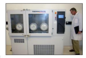
The test chamber includes two separate, independently controlled test spaces: one compartment for conditioning
