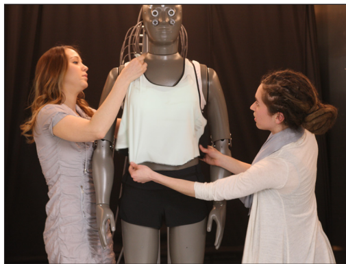
Two faculty members prepare a Thermal Manikin for a temperature and humidity environmental test in the Thermotron Walk-In Chamber.
