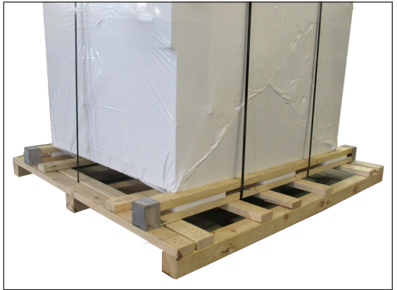
Thermotron's new pallet design uses thick, dense foam between wooden boards with metal end caps to help reduce the amount of shock during transport.
