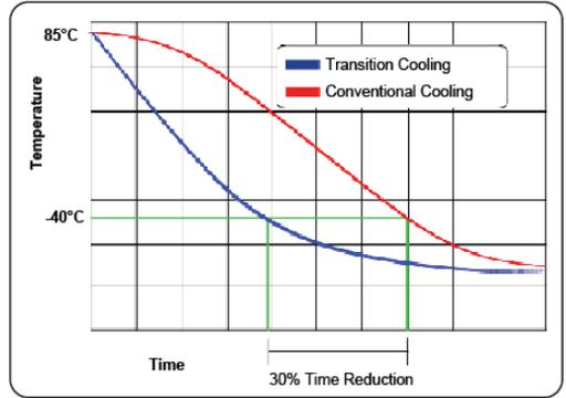
This innovative feature increases ramp rates up to 30% while reducing power consumption, as shown in the graph above.
