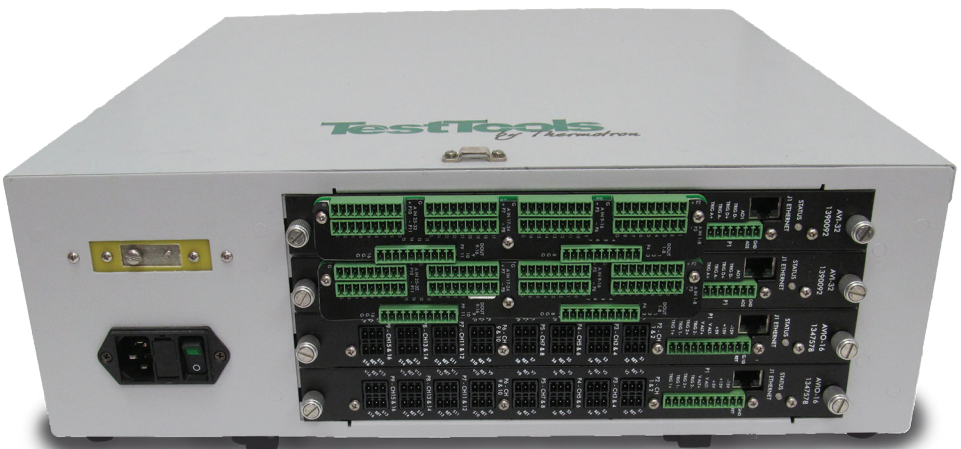
4 Slot Chassis with 2 AVI and 2 AVIO Boards
