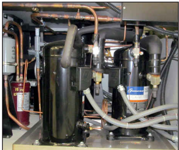
Refrigeration section of a refurbished, nearly new Thermotron chamber.
