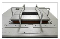
Releases when pressures are too great. A metal cage houses the blow-off top to block particulates from escaping the chamber.
