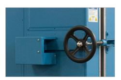
A heavy-duty door handle ensures that pressures will not blast the door open.
