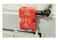
Prevents access to the testing chamber during a normal cycle or when an alarm condition has been detected.
