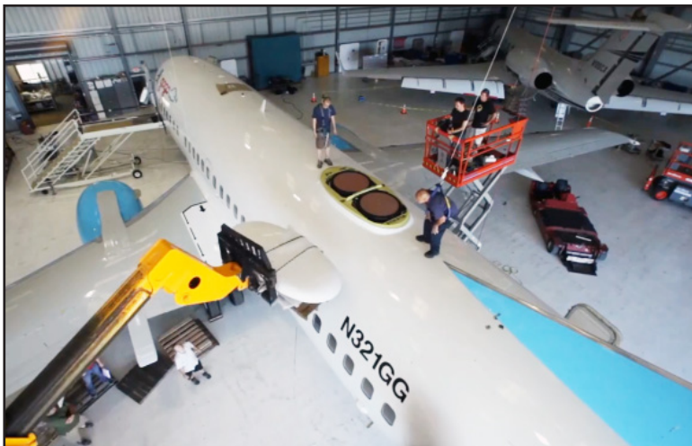
ThinKom's low-profile antennas are the industry leaders in providing in-flight Wi-Fi to commercial airline passengers. Pictured is one of ThinKom's signature Ku-Band antenna systems being installed atop a commercial aircraft.
