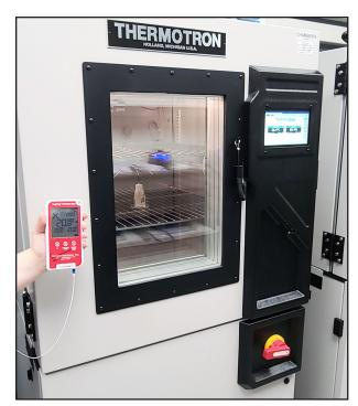
A Thermotron at work, ensuring a Control Solutions vaccine data logger is correctly measuring the environment of the test subject within the chamber.
