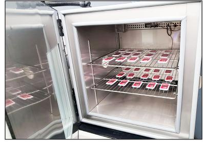
Thermotron's consistent performance across the entire chamber is ideal for Control Solutions testing and calibrating numerous data loggers at once. The air flow design within the S-Series chambers ensures there are no hot or cold spots or inconsistent humidity levels that could negatively impact the calibration process.
